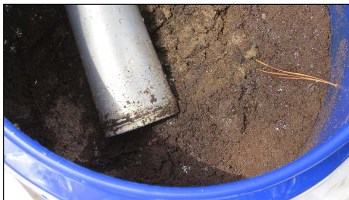
Figure 3.1—Target 9% Oil in Sediment Mix
