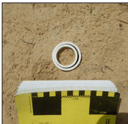
Figure 3.8—“Target” Tube Loaded in “Outer” Tube
