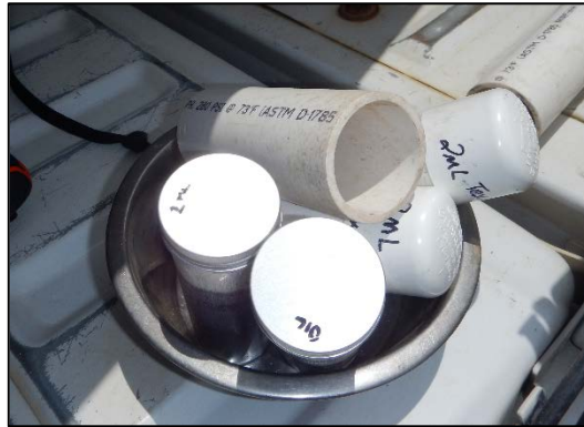
Figure 3.3—Inner and Outer PVC Pipes for the Wide Area Search Tests
