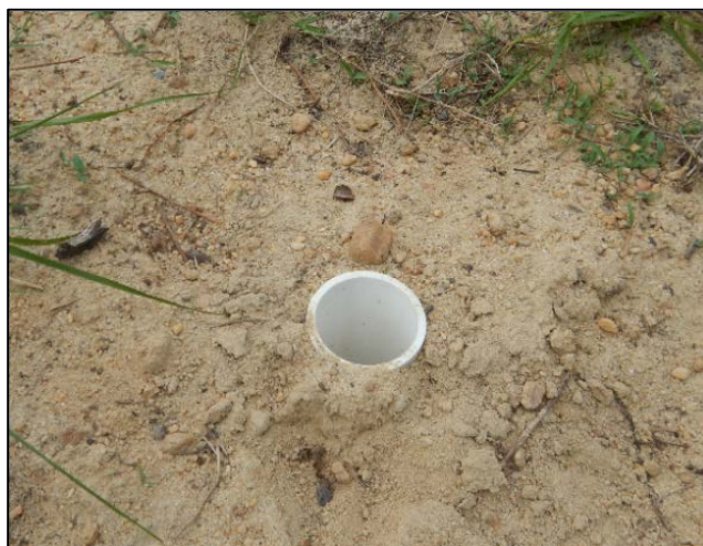
Figure 3.6—Buried “Outer” Tube
