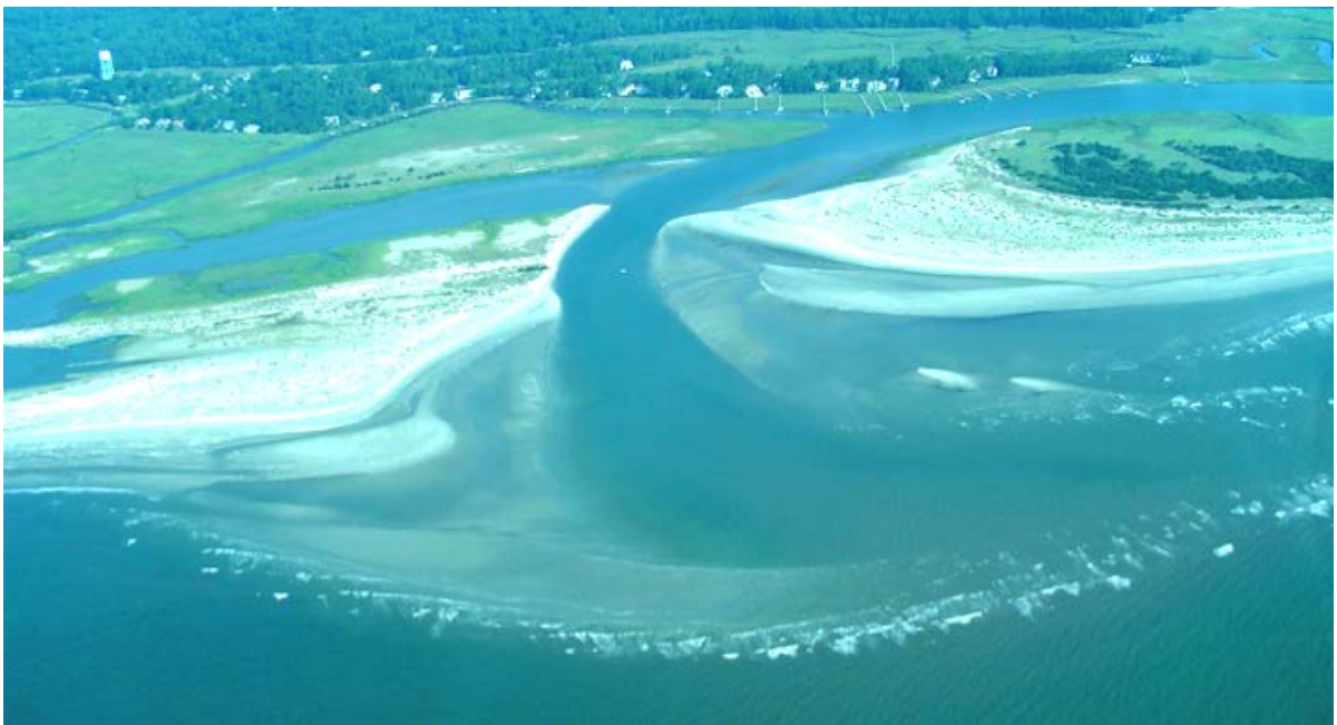
Figure 2.5. Oblique Photograph of a Mixed-Energy Inlet
