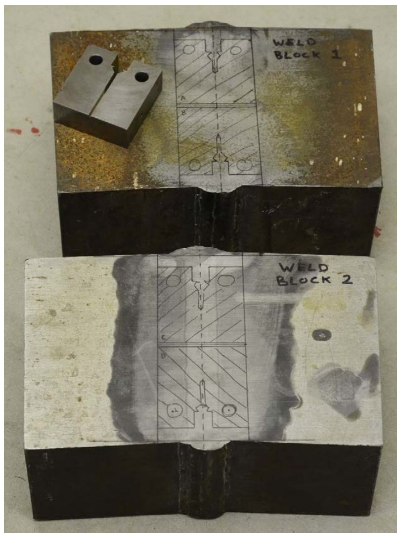
Figure 8—C(T) specimen orientation in the welded blocks of 2½Cr-1Mo-¼V steel.
