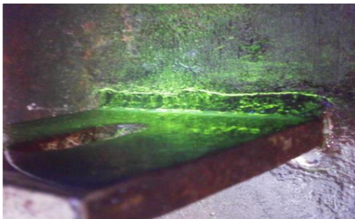
Figure 4—Cracking On the External Surface at an Insulation Clip Displayed by Wet Fluorescent MT
