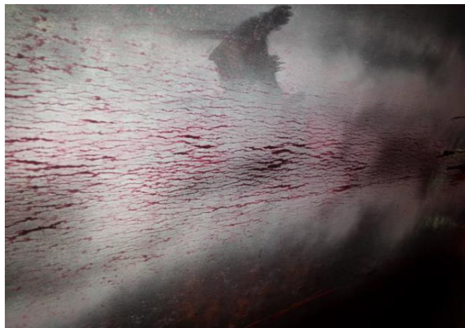
Figure 3—PT from the Outside Surface Displays an Area with “Elephant Skin” Cracking
