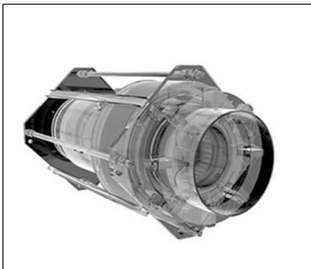
Figure 7—Cold Wall Refractory Lined Expansion Joint with Bellows Protected and With Erosion-resistant Refractory and Hexmetal on Steel Sleeves
