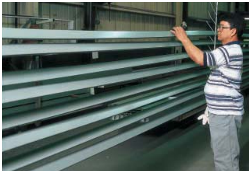
Testing thickness and color quality of painted finish
