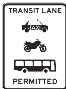
FIGURE 1 EXAMPLE OF A TRANSIT LANE INFORMATION SIGN
