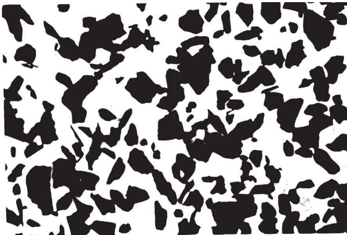
FIGURE 4 SHAPE AND SIZE—UNACCEPTABLE CHARACTERISTICS
