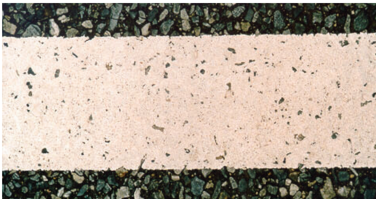
FIGURE L1 95% OF AREA INTACT
