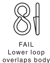
FIGURE 2.2 EXAMPLES OF CONNECTING DEVICES THAT PASS AND FAIL THE REQUIREMENTS FOR CONNECTING DEVICES
