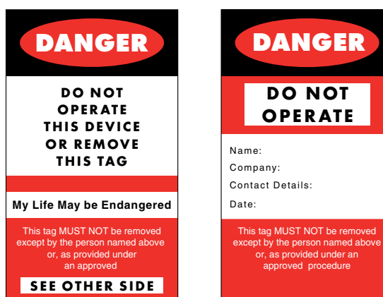
Figure 3.1(C) — Typical danger tags
