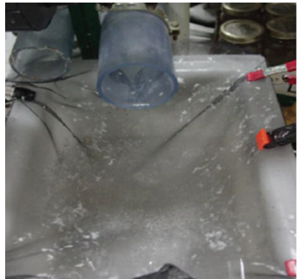
(f) Drain line outlets with screen to collect flushed materials
