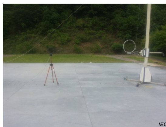
b) Measurement at coplanar direction at 3 m
