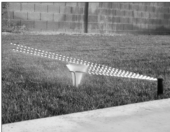
Figure 4 – Incorrect placement of catch device
