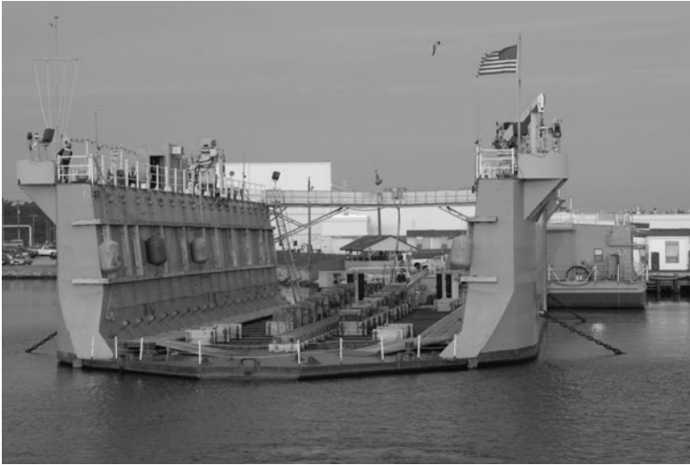
Figure 1-1. Floating dry dock. Source: U.S. Navy photo by Mass Communication Specialist Seaman Kelly E. Barnes.
