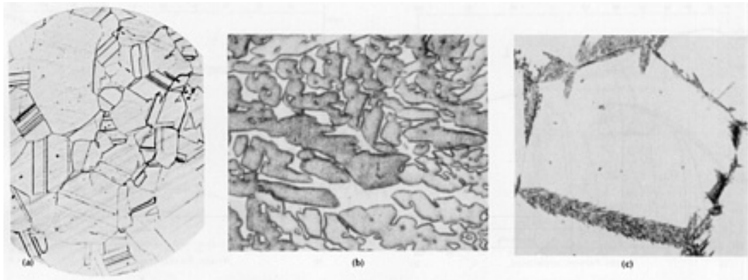
Fig. 41 The microstructures of two common brasses. (a) C26000 (cartridge brass, 70%), hot rolled, annealed, cold rolled 70%, and annealed at 638 °C (1180 °F), showing equiaxed grains of copper solid solution. Some grains are twinned. 75×. (b) C28000 (Muntz metal, 60%) ingot, showing dendrites of copper solid solution in a matrix of \beta . 200×. (c) C28000 (Muntz metal, 60%), showing feathery of copper solid solution that formed at \beta grain boundaries during quenching of the all- \beta structure. 100×. Source: 85ASM 13
