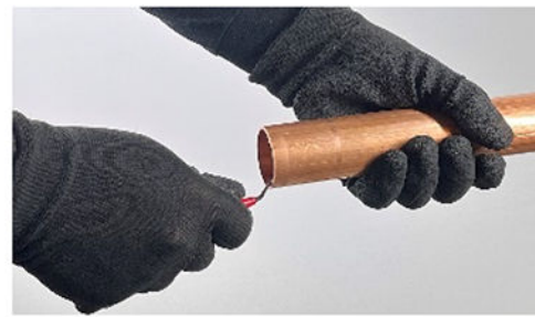
FIG. 5 Reaming Blade on the Tube Cutter, Half-Round or Round Files (left) and Pen Reamer (right)
