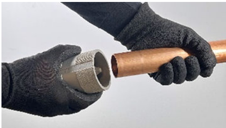
FIG. 3 Remove Any Burrs on the Outside of the Tube Ends
