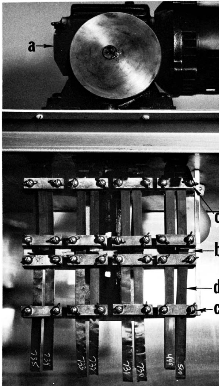
a—gear head and eccentric drive b—traveling bar with specimen clamps, driven through roof of ozone chamber c—stationary bars with specimen clamps d—specimens
