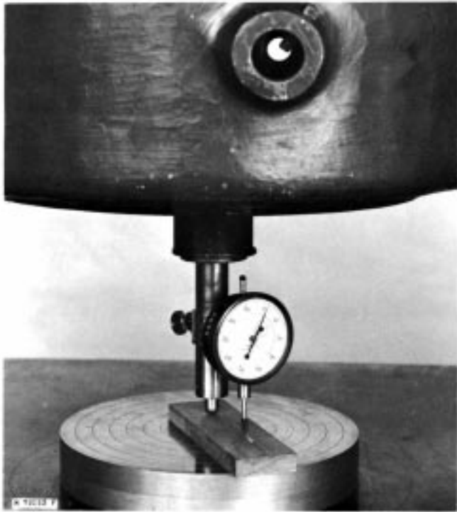
FIG. 1 Apparatus for Hardness-Penetration Test
