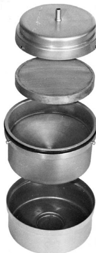
FIG. 1 Pressure Bleeding Test Cell A
