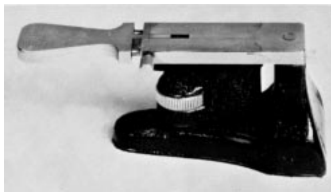
FIG. 1 Heavy-Duty Cross-Section Device
