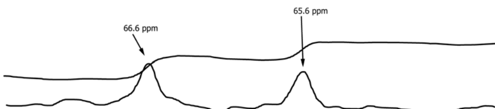
FIG. 4 Secondary Hydroxyl Carbon Peaks of 5500 MW Triol (78 % Primary)
