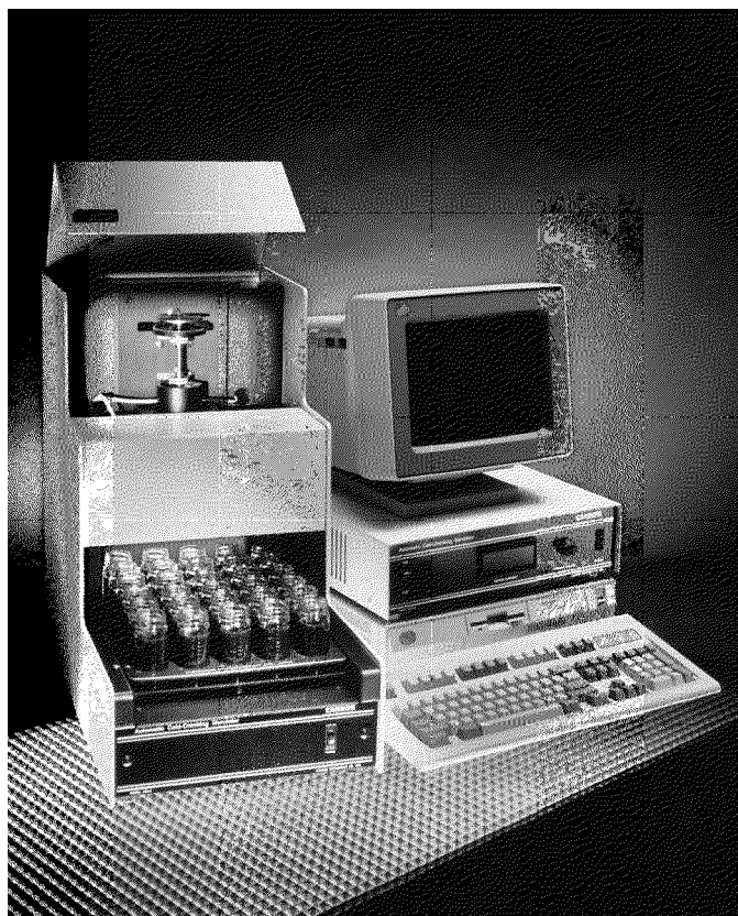
FIG. 3 Automatic Automated Cold-Cranking Simulator
