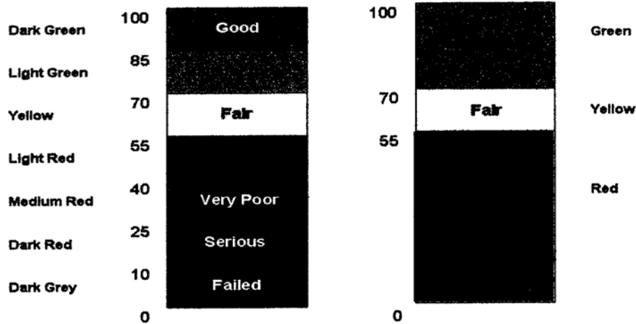
FIG. 1 Two Examples of Pavement Condition Index (PCI (trademarked)) Rating Scales
