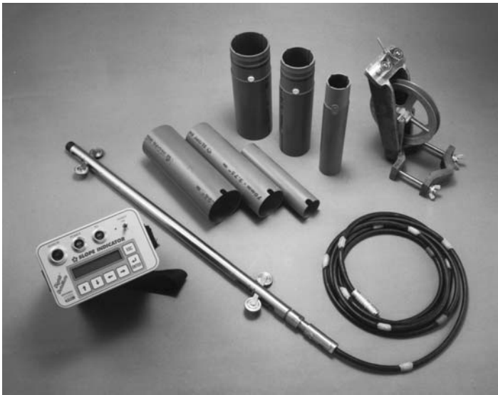
FIG. 1 Typical Components of Inclinometer System
