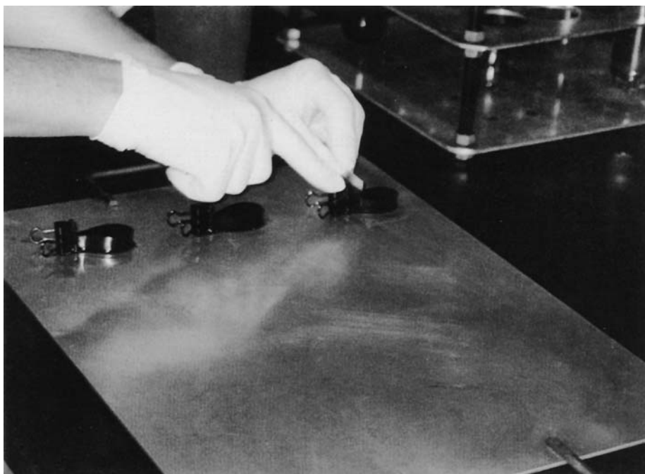
FIG. 1 Placement Binder Clips with Rubber Specimen on the Aluminum Plate
