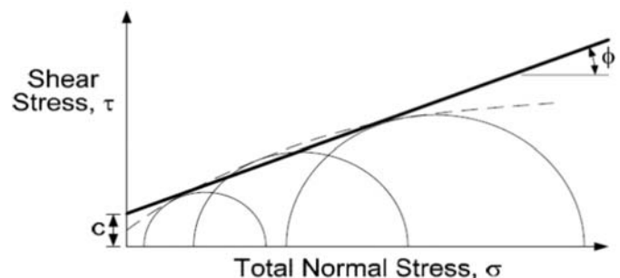
FIG. 1 Curved Mohr failure envelope and equivalent Mohr-Coulomb linear representation (from Figure 20.16)
