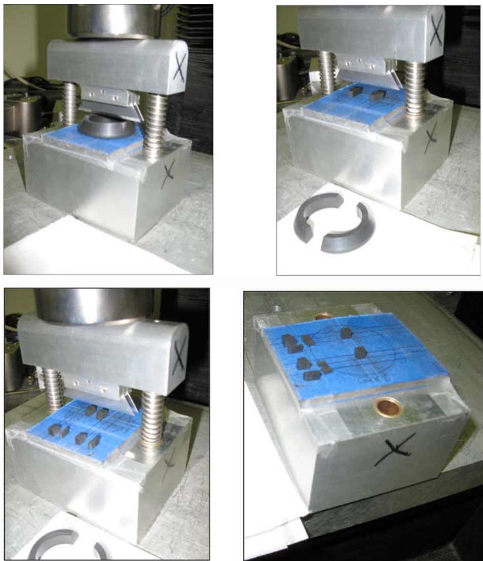
FIG. 1 Typical Die and Cube Cutting Sequence
