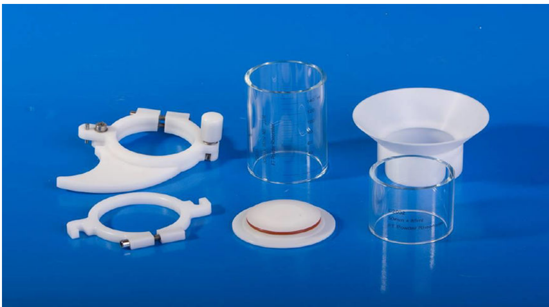
FIG. 5 Components to Assemble the 50 mm x 160 mL Split Vessel (4mm ball-ended hex key not shown)
