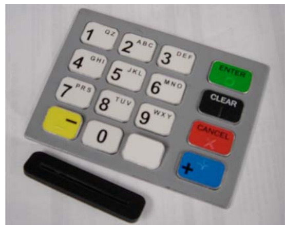
FIG. 8 Example of Keypad Overlay
