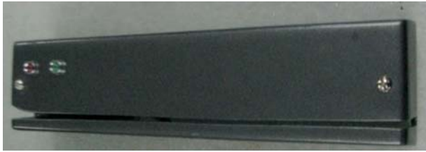
FIG. 5 Example of a Custom Skimmer (Door)
