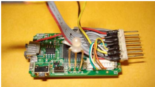
FIG. 2 Example of an Altered Hand-Held Skimmer
