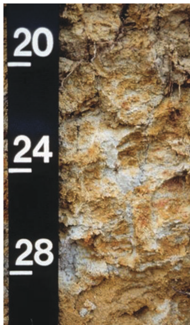
NOTE 1—Photo is courtesy of USDA Natural Resources Conservation Service. FIG. 1 Example Orange-Brown Soil Matrix Interspersed With Grey Mottles
