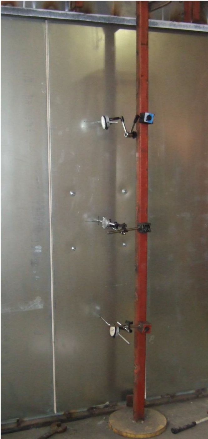
FIG. 1 Setup to Measure Deflection
