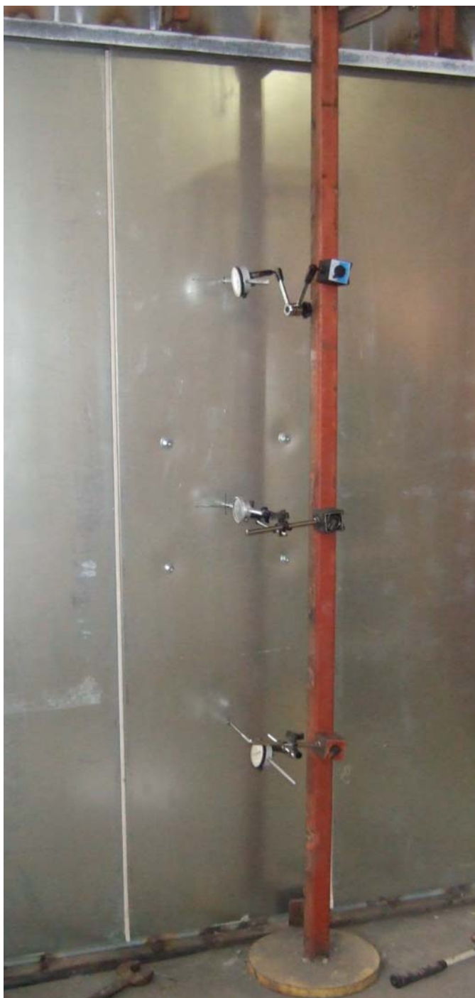
FIG. 1 Setup to Measure Deflection
