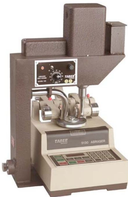
FIG. 1 Taber Abraser with Grit Feeder
