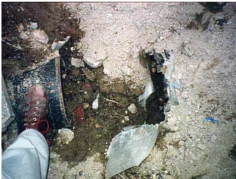
Figure 2-5B Ductile-iron joint pulled apart due to lateral spreading
