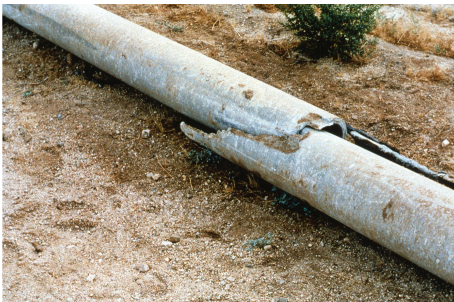
Figure 2-3B Landers–Big Bear earthquake pipe broken in the fault offset
