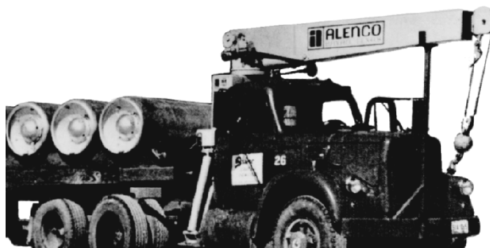
Figure 4-3 Chlorine ton container truck
