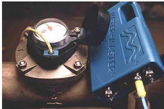
Figure 3-1 Meter Master EL 100 flow recorder and water meter
