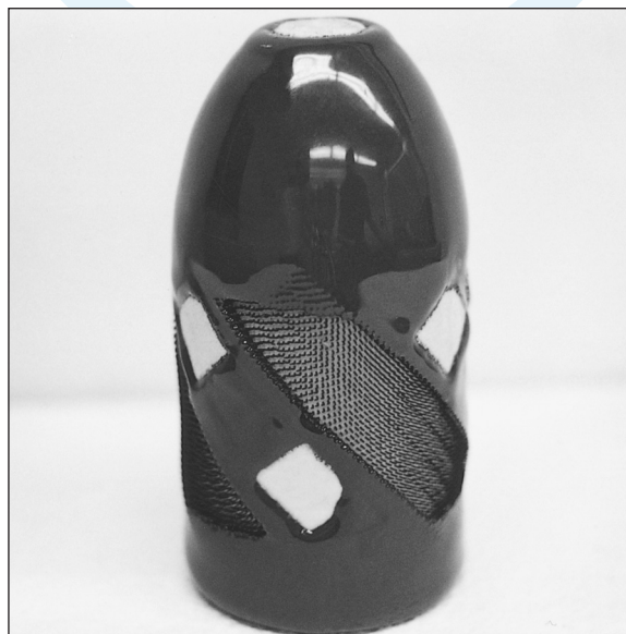
Figure 4-3 A foam pig with hardened coatings
