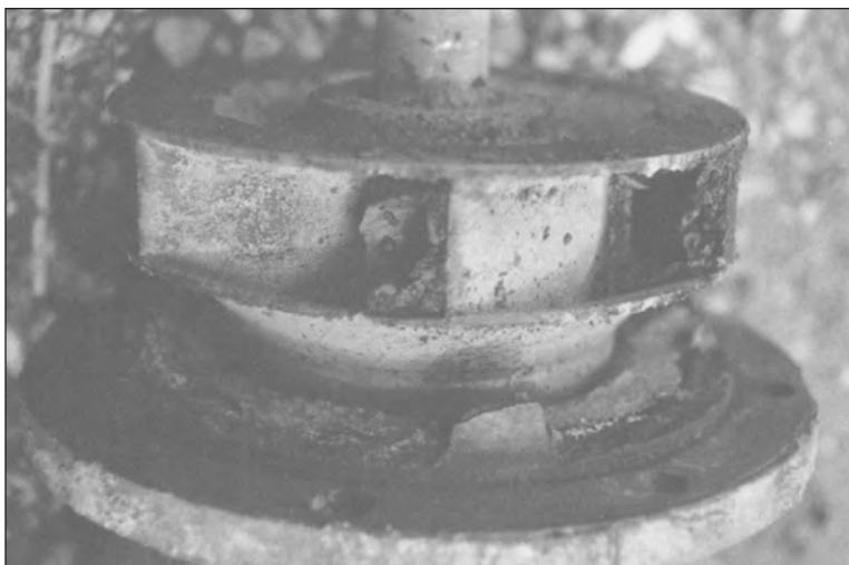
Figure 2-6 Partly filled impeller channel
