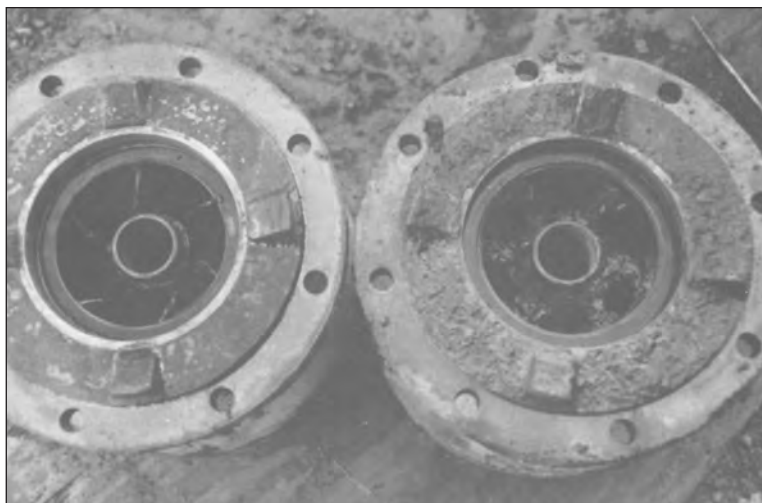
Figure 2-9 Clean versus clogged impellers
