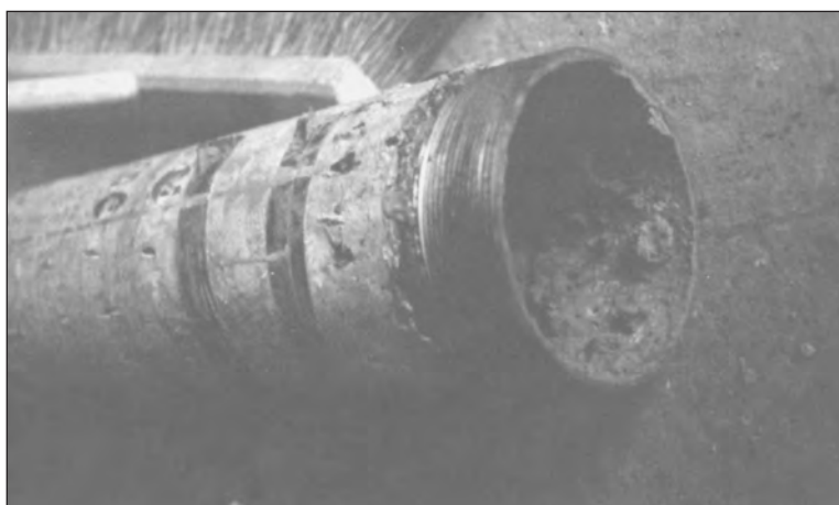
Figure 2-8 Column pipe with iron biofilm
