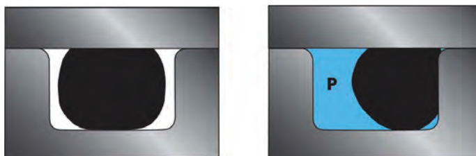
Figure 2-3 O-ring installation without and with pressure (P)
