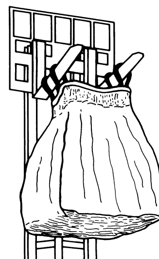
(b) Flexible IBC fitted with slings
