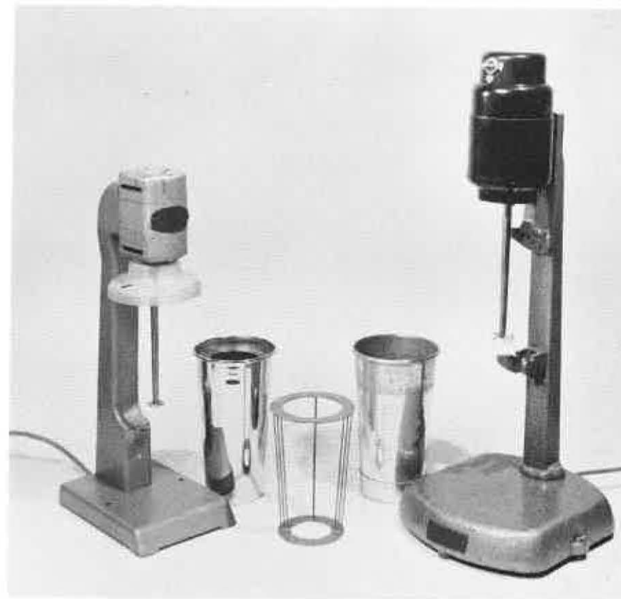
Fig. 12. Two types of stirrer suitable for use in the fine particle size analysis
