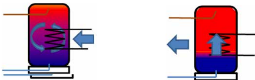
a) Charging phase of a mixed storage system b) Discharging phase of a mixed storage system
