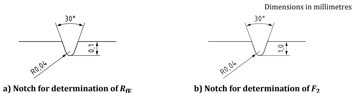
Figure 3 — Fatigue test piece notches
