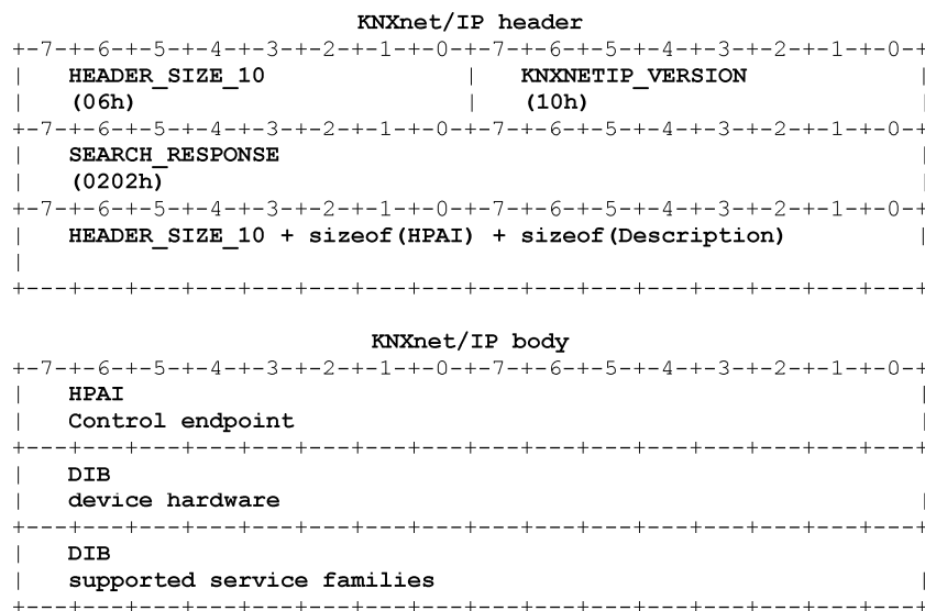
Figure 18 — SEARCH_RESPONSE frame binary format
