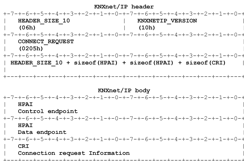
Figure 21 — CONNECT_REQUEST frame binary format
