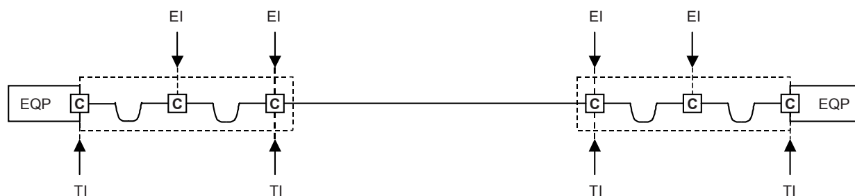
Figure 5 – Test and equipment interfaces for backbone cabling
