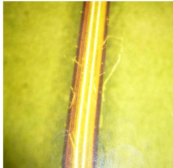
Figure A.2 – Surface enamel peeling like string
