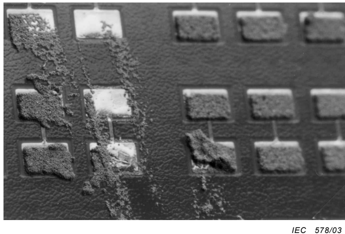
Figure 5 – Smudged paste – Nonconforming
