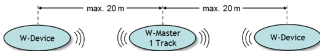
Figure 8 – Radius of a cell with a 1 W-Track W-Master
