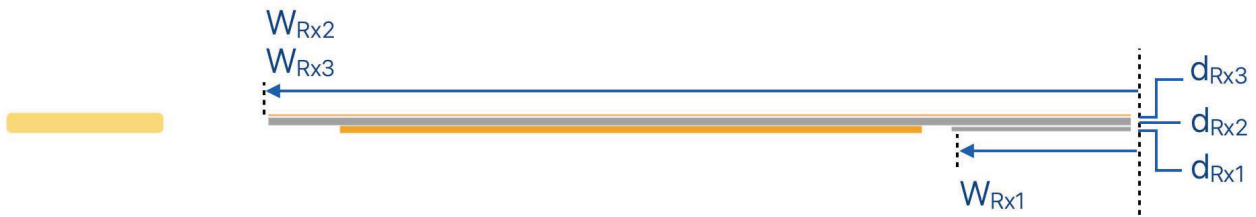
Figure 4.3.1.4: 19 Cross-section of the coil module for the PRx coil system model.
